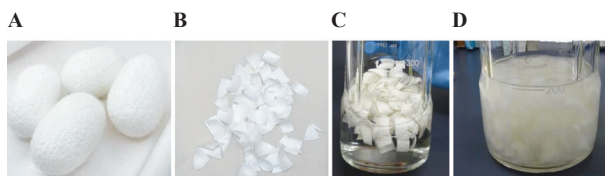
Figure 1 Extraction of sericin(High-pressure steam sterilization method) (a) Silk cocoons. (b) Cut silk cocoons into 1 cm squares. (c) Cut cocoons with distilled water in a medium bottle. (d) After autoclaving at 121℃ for 20 minutes.
